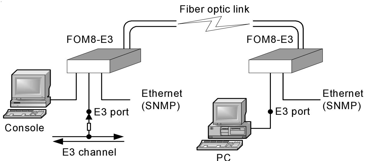
In the monitoring mode, the E3 receiver is connected via external resistor to the required line of the E3 channel, and the E3 transmitter is switched off. Signal attenuation in the resistor is compensated by additional gain. The received data may be sent to a PC for processing (the Cronyx Tau-PCI-E3 board may be used).
