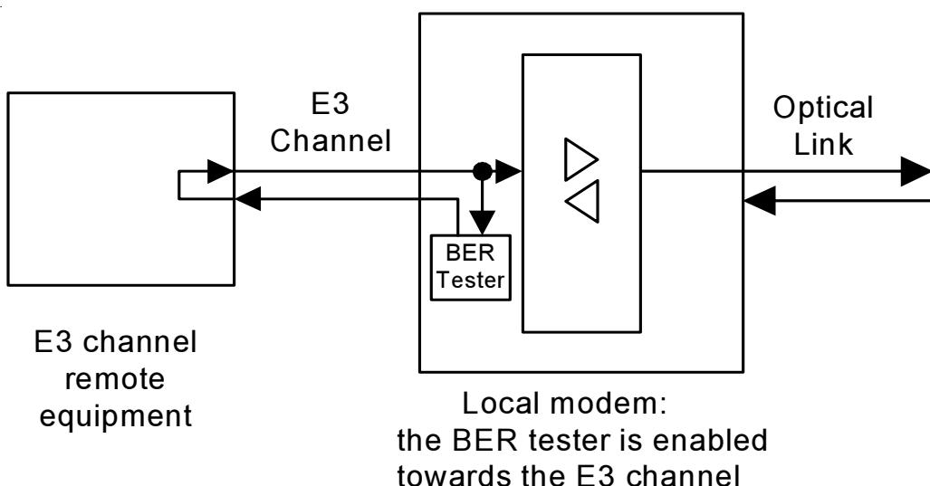
Testing is performed using the full bandwidth. On the remote equipment of the E3 channel, a loopback must be enabled towards the E3 channel.
