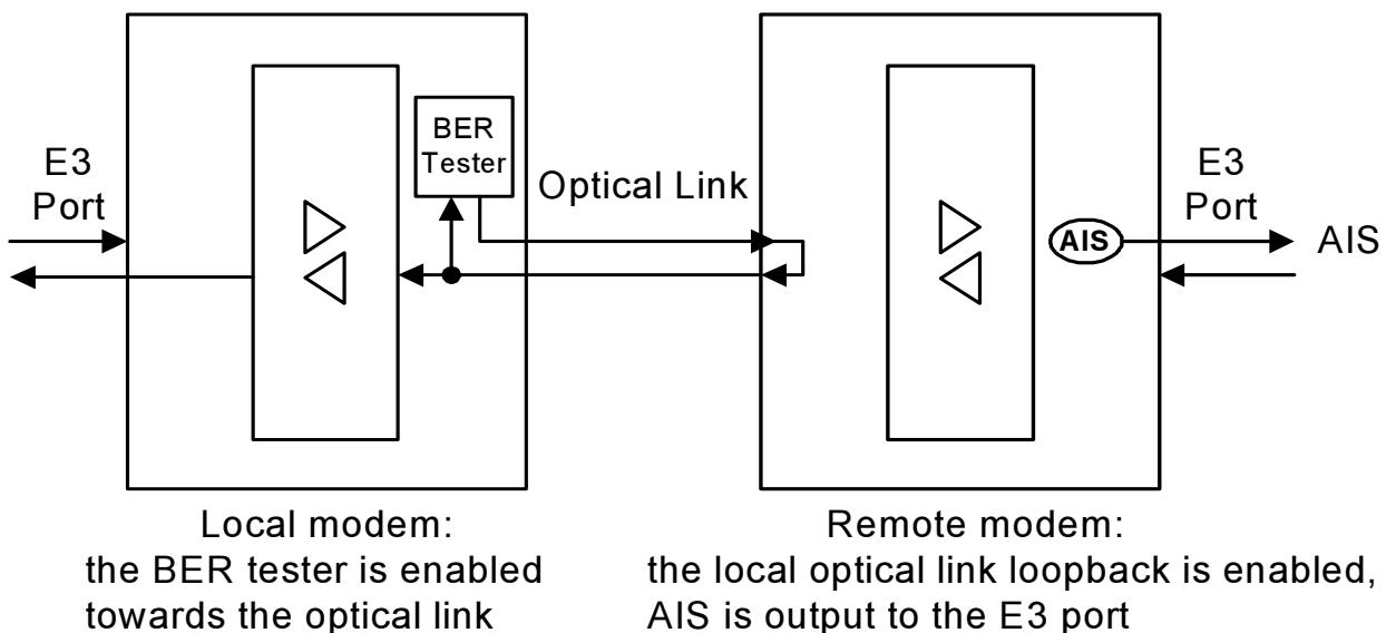
If the devices operate in the Framed mode, the testing does not violate framing, and the capability to control the remote device from the console of the local device is preserved. When operating in the Transparent mode, testing is performed using the full bandwidth of the optical link.
