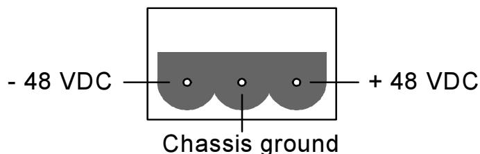
The 3-screw removable terminal block is supplied with the device.
