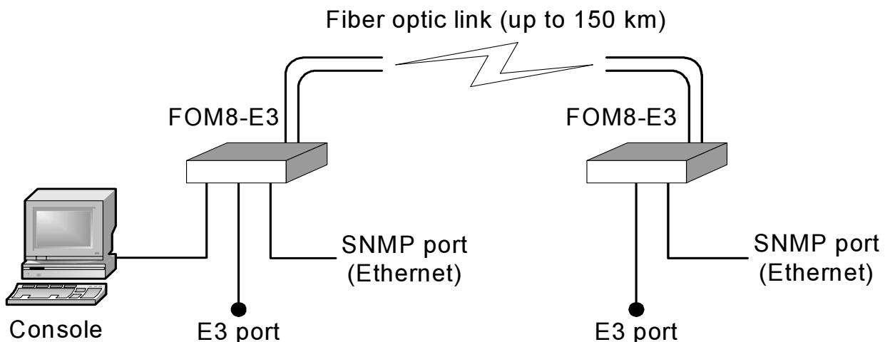
The FOM8-E3 operation may be controlled from the ASCII terminal (*the console*) connected to the FOM8-E3 control RS-232 port or from Ethernet network by the SNMP protocol.
