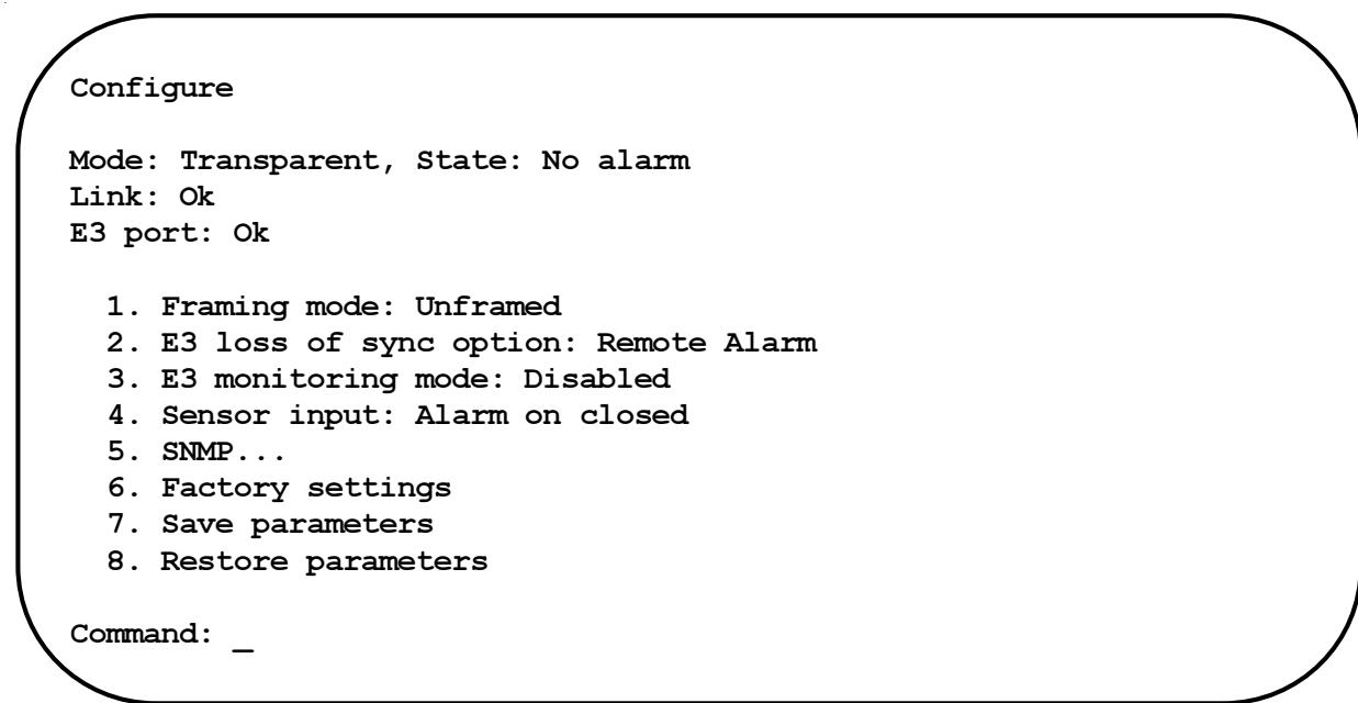
Use the «*Factory settings*» command to return parameters to their default values (for details see the appropriate section below).
